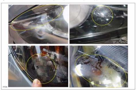
This concern is caused by gas that emits from a gasket in the lamp unit. The gas adheres to the inner surface of the headlight lens and reacts with the anti-clouding coating and moisture in the air to create white milky stains.
